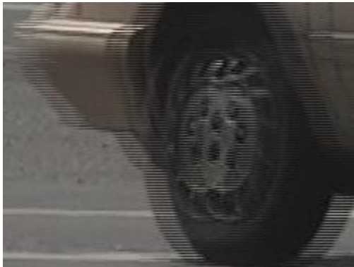
An example of interlaced video showing a wheel of a moving car.
